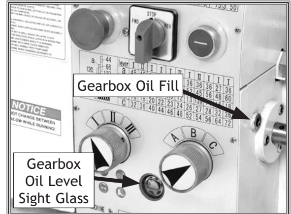
Figure 36. Headstock oil level sight glass.
